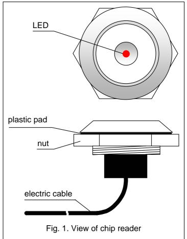
In order to get access, put the chip into the reader recess to close the electric circuit. The reader will read the chip code and the alarm control panel will react according to the preprogrammed function and authority level of the user of the particular chip, e.g. it will release an electromagnetic door lock.
